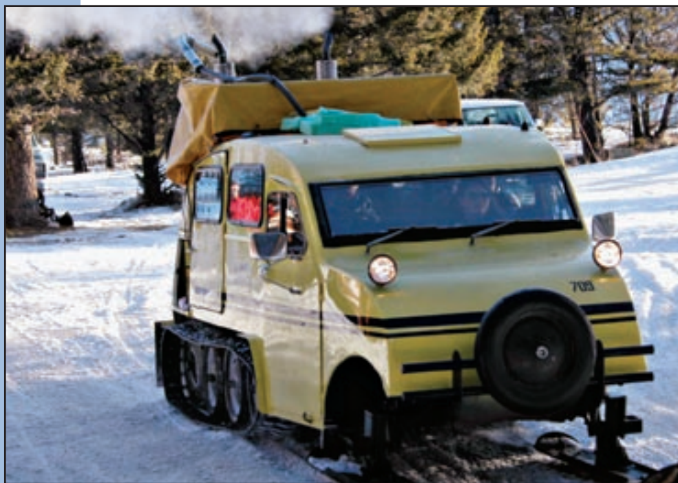
Over the snow and through the woods. A vintage Bombardier snowcoach showing the heated exhaust probe inserted in the passenger-side exhaust pipe.
