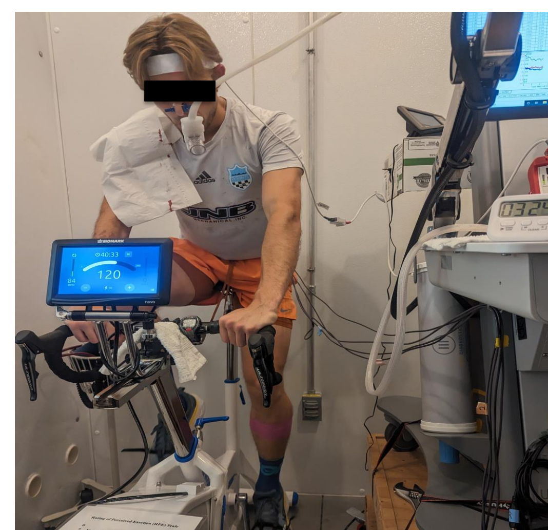
Chamber Set-Up: Upright cycle ergometer and metabolic cart. Subject completing ventilation and gas exchange measurements.
