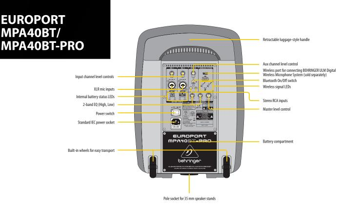
Note: MPA40BT is functionally the same as the MPA40BT-PRO without the retractable luggage-style handle and wheels.
